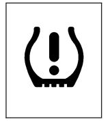
This light will come on briefly as you start the engine, for vehicles equipped with the Tire Pressure Monitor System.
